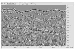
Figure 10. The stacked migration using the true velocity model.
