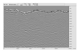
Figure 5. Stacked migration from the initial velocity model.
