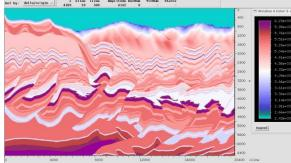
Figure 9. The true velocity model derived from Canadian Foothill. This model is used to generate synthetic seismic shots for this study.
