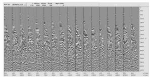
Figure 6. The common image gathers for every 100 xline using the updated velocity model from the proposed joint tomography after several iterations.
