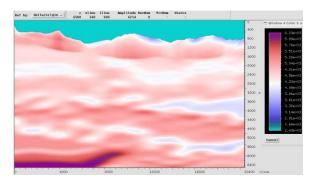
Figure 3. The combined initial model for reflection tomography. Inverted near surface model from turning-ray tomography.
