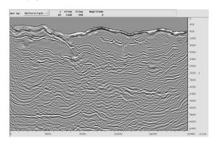
Figure 7. The stacked migration using the updated velocity model from the proposed joint tomography after several iterations.
